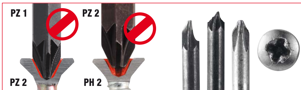
Screwdriver-to-fastener torque transmission.
