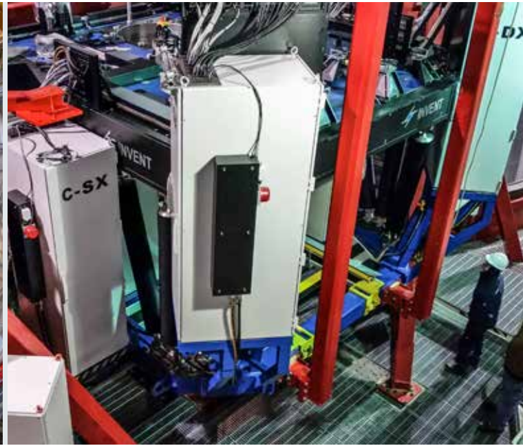
The LINC-NIRVANA astronomical instrument was built and tested at the Max Planck Institute of Astronomy in Heidelberg, Germany. The right picture shows the instrument mounted on the telescope platform at LBT in Arizona with white electronic cabinets and black carbon fibre structure.
