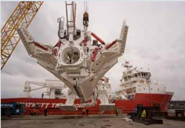
It is part of a complex and precisely choreographed process for protecting, stabilizing and insulating oil and gas pipes under the sea; a 'rigid' concrete-clad pipe is laid directly onto the seabed by a pipelay vessel, to be then buried by the pipeline plough which digs the trench beneath the pipe as it is pulled along the pipe route on the seabed. A backfill plough then scoops back the excavated soil to cover the pipe.
